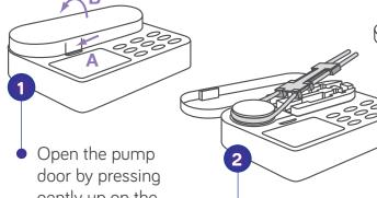
Open the pump door by pressing gently up on the lower wall (A) and rotating the door upwards (B) at the same time.
